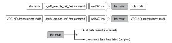
Figure 13 Process flow for performing the built-in self-test.
