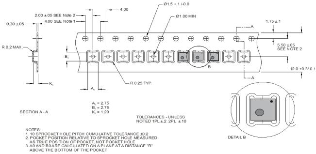
Figure 20 Technical drawing of the packaging tape with sensor orientation in tape. Header tape is to the right and trailer tape to the left on this drawing. Dimensions are given in millimeters.
