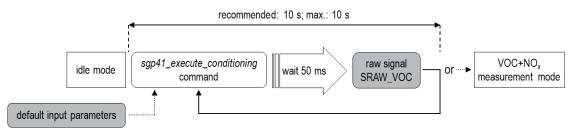
Figure 8 Optional process flow for executing the conditioning of SGP41 and reading out the VOC raw signal.
