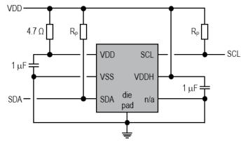
Figure 6 Typical application circuit.
