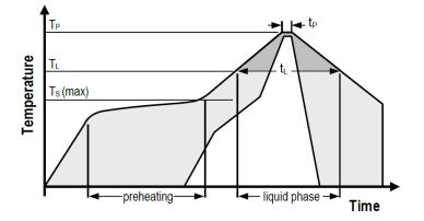
**Figure 19** Soldering profile according to JEDEC standard. Recommended conditions are  $T_P = 245^{\circ}C$  and  $t_P \le 30$  s for Pb-free assembly,  $T_L < 220^{\circ}C$  and  $t_L < 150$  s. Ramp-up rate  $<3^{\circ}C$  s<sup>-1</sup> and ramp-down rate  $<4^{\circ}C$  s<sup>-1</sup>.
