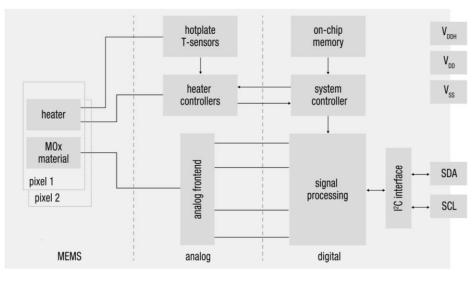
Figure 1 Functional block diagram of the SGP41.
