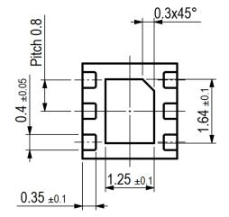
Figure 17 Package outline drawing of the SGP41. Dimensions are given in millimeters.
