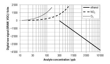
**Figure 2** Typical sensor response by the VOC signal to ethanol, NO<sub>2</sub>, and O<sub>3</sub> normalized to 500 ppb of H<sub>2</sub> + 500 ppb of ethanol. Data were recorded at 25 °C and 50 % RH and a power supply of VDD of 3.3 V.
