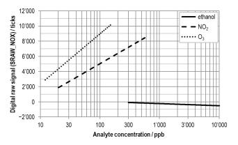
**Figure 3** Typical sensor response by the NO<sub>x</sub> signal to ethanol, NO<sub>2</sub>, and O<sub>3</sub> normalized to 500 ppb of H<sub>2</sub> + 500 ppb of ethanol. Data were recorded at 25 °C and 50 % RH and a power supply of VDD of 3.3 V.
