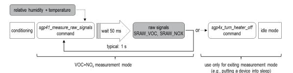
Figure 9 Process flow for performing a raw signal measurement with the SGP41. For enabling on-chip humidity compensation, current relative humidity and temperature values have to be supplied as part of the measurement command.
